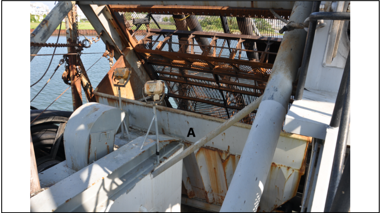
A view of the underside of the dredge on the gantry from gantry superstructure. The dredge is low on the structure in this image, the large hopper into which the dredge empties is marked A.
