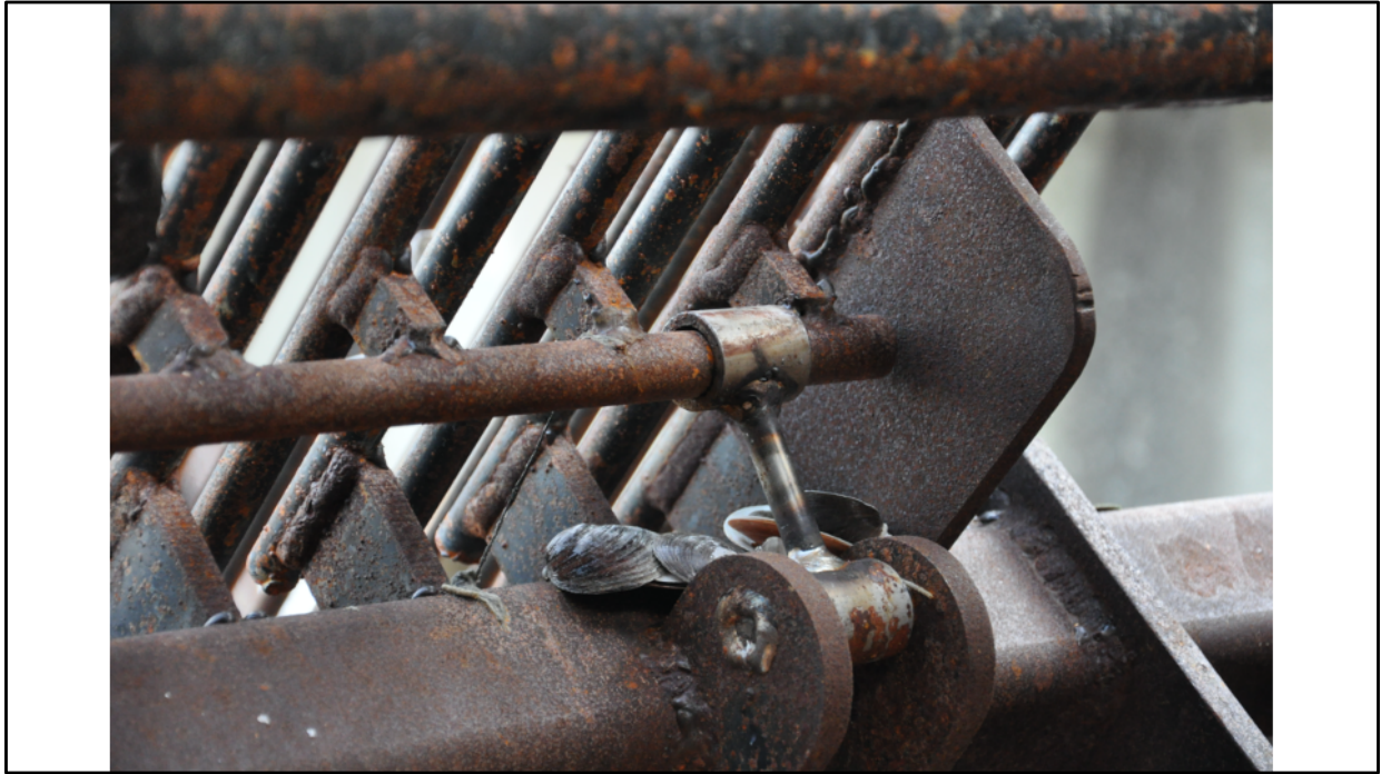
This close up shows the mounting points of the alternating bars.
