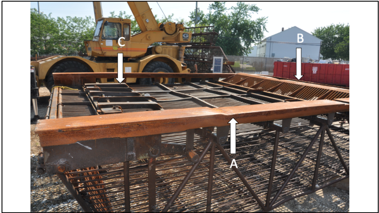
This view of an inverted dredge in the shipyard shows the runners (A), position of the knife (B) to the right (front of the dredge) and the door at the rear of the bottom of the door (C) that opens a the dredge is hauled up the gantry on retrieval.
